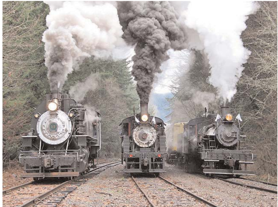
The Mt. Ranier Scenic Railroad near Mineral, Wash., has restored three locomotives from the '20s.. From left, Hammond Lumber Company No. 17, an Alco 2-8-2T built in 1928; Hillcrest Lumber Company No. 10, a 3-truck Climax built in 1928; and Pickering Lumber's 3-truck Pacific Coast Shay vintage 1929. The locomotives pull passengers through the foothills of Mt. Ranier. To learn more, visit www.mrsr.com .
